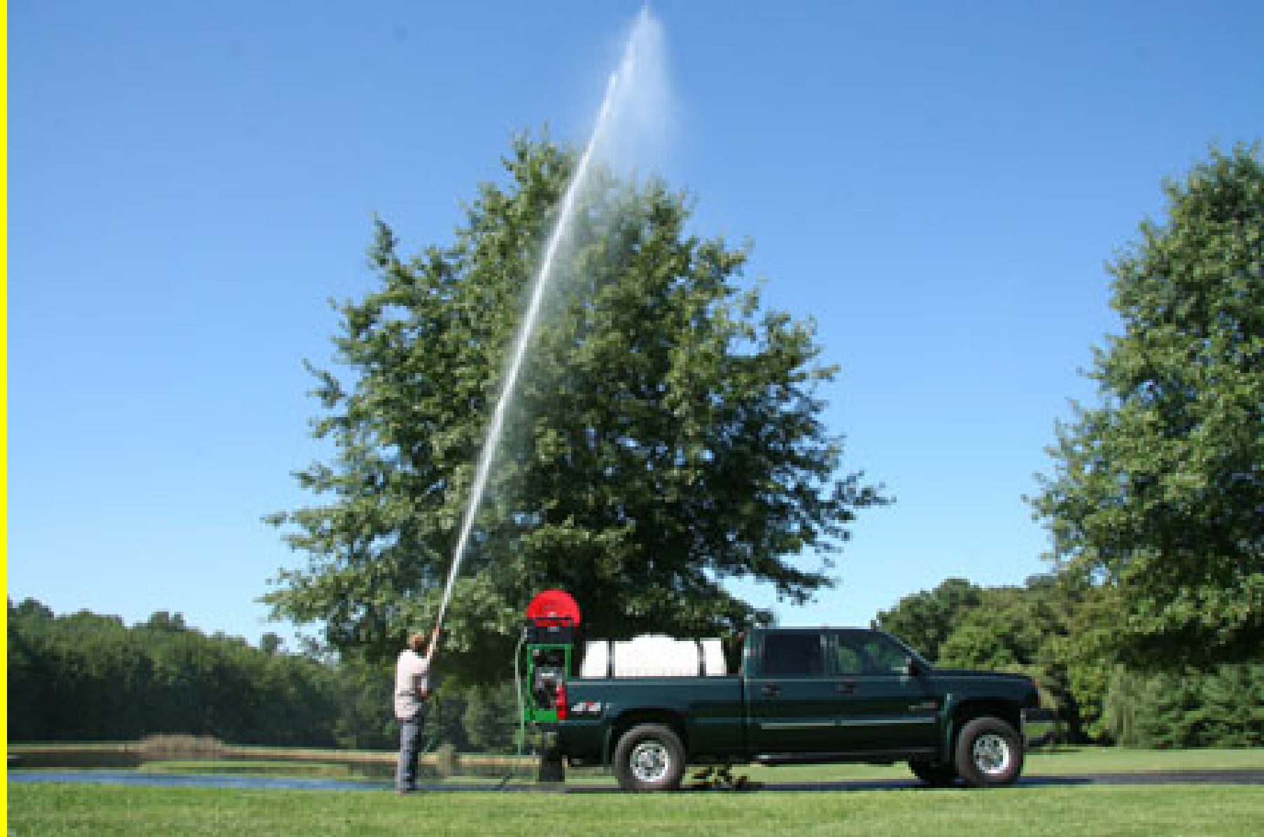
42 gpm 700 psi tree sprayer
