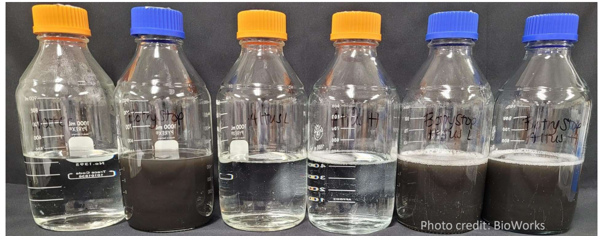
Compatible, last two mix bottles look homogenous and no difference to controls
